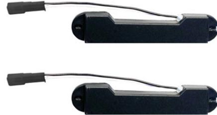
The iKey uses a sophisticated Dual Zone antenna system to allow it to effectively operate on everything from a small sub-compact to full size SUV, the systems dual antenna design guarantees consistent range and performance regardless of vehicle type. The Main Antennas generate a low frequency RF field that extends approximately 4 feet around the vehicle. When you enter this field, the low frequency RF signal triggers the iKey Fob in your pocket to transmit its authorization code to the system.
