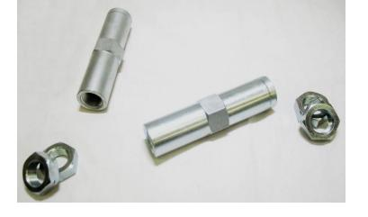
Optional billet adjuster sleeves in above picture. You will not need to re-use your inner tie rod links. Inner tie rods are included, outer tie-rods are not included.
