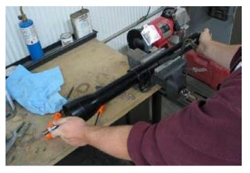
Next mate the universal shafts to the upper shaft. This is easier to accomplish on a bench as shown than trying to assemble this in the car.
