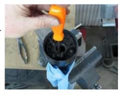
Then pull the switch assembly out of the way and removed the old steering column upper bearing and test fit the new bearing in the hole. Note that some applications require the reuse of the original bearing outer race.
