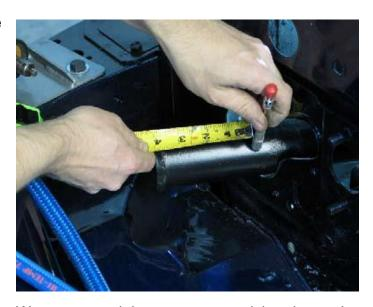
We recommend that you use a straight edge and mark the column on the underside where it intersects the firewall and come out ¼-inch for your cut line. This allows you to measure twice and cut once.
