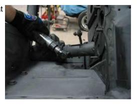
the shaft. This will allow more "wiggle" room for the steering box removal. It is also a good Idea to wrap the steering shaft in towels to prevent damage to the interior.
