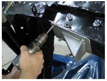
Use a 3/8-inch drill bit to bore the two per side outer mounting holes in the frame rail lip.
