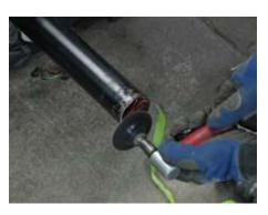
Make sure of your mark and remove the column. Measure the distance from the end of the column to the mark and repeat the mark around the column Use an awl or endurable marker to scribe mark lines. Place tape around the column to aid in cutting the end off as shown A cut-off wheel
