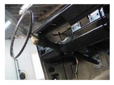
Installation is almost complete. Check rack for ease of movement; there should be no binding in the universals. Use a mirror to check for any contact between the bearing flanges. If they are where they should be the rack should operate smoothly. You may experience some "soft" binding from the collapse of the bellows as the wheel is turned—this is normal. Any hard binding should be worked out by movement of the shafts.
