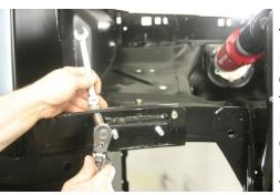
The bolts are installed and tight ened. They are used to triangulate the load of the brackets giving a good, strong mounting point for the rack.
