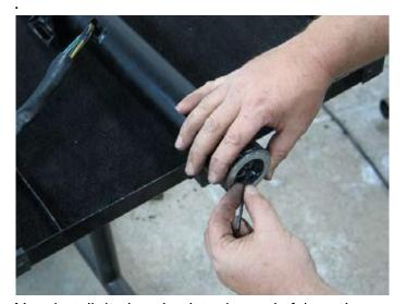
Next install the bearing into the end of the column. The bearing is held in place by three Allen head screws.
