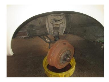
Remove the front wheels to allow easy access to the steering components. If you are only, installing a rack it is not necessary to remove the original suspension. How ever since we are installing a strut kit on this application, we will be removing the entire assembly as a unit.
