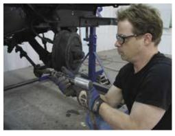
A narrow tie rod splitter makes short work of the outer tie rod removal. It is recommend ed that you replace the
