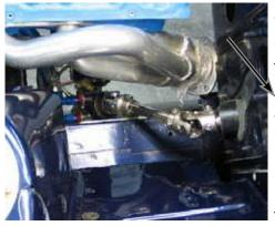
Attached the lower universal joint to the steering head of the rack and push the top universal into the column until there is no binding in the joints. Leave the lower column mount
