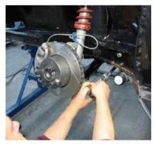
Install the adjuster sleeves. Start both the inner and outer tie-rod ends at the same time to assure equal deployment on the adjuster.
