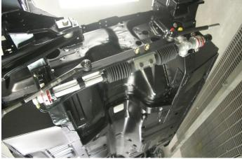
The basic rack is now installed on the chassis. Check fit and clearance of the rack.
