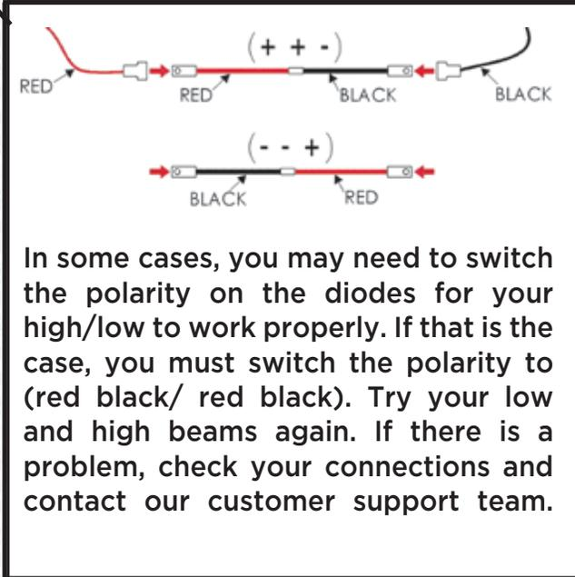
In some cases, you may need to switch the polarity on the diodes for your high/low to work properly. If that is the case, you must switch the polarity to (red black/ red black). Try your low and high beams again. If there is a problem, check your connections and contact our customer support team.
